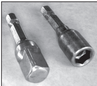
Photo 5: Drill socket driver for 3/8" sockets and 5/16" nut setter for hose clamps.
