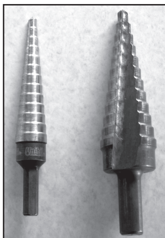
Photo 4: Step drill bits. The one on the left goes from 1/8" to 1/2". The one on the right goes from 3/16" to 7/8".
